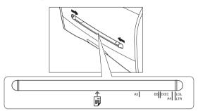
Insert the paper straightly into the multi-purpose feeder with the print side up.
